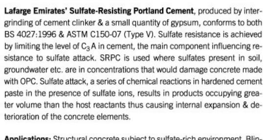
**Applications:** Structural concrete subject to sulfate-rich environment, Blinding / PCC, Sewage treatment structures, Mass concrete structures, Piles, Foundations, Underground structures, Precast concrete etc.
