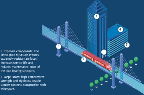
cross-sections require less valuable space, thus increasing the usable area. 4. **Slabs:** reduced thickness allowing
